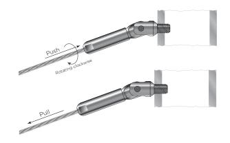
**9.** Feed bare end of cable through intermediate posts towards tensioning fitting on opposite end of frame, mark cable at score mark on body of the tensioning fitting. Cut cable at this mark.
