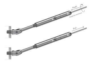
Tension cable by holding Push-Lock<sup>®</sup> body at 3/8" wrench flat nearest cable (do not let this section rotate while cable is inserted) and tightening female threaded section of fitting with a 3/8" open end wrench.
