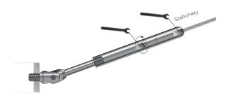
**12.** Tension all cables to desired amount. It is best to start tensioning at the top and bottom cables of your panel and work in an alternating pattern towards the center of the panel (see illustration).
