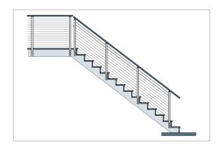
F1. Handrail must be mounted prior to cable infill installation. Complete the railing by adding infill. Please refer to <u>Installation Instructions for Metal Posts</u> on Stair Runs, Tensioning
