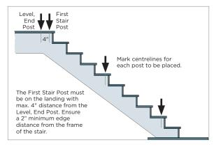
D1. **Post Spacing:** Using 40" on center as the maximum spacing between posts, determine where each post will be placed and mark their centerlines. Do this for the entire level run of your project. Spans greater than 40" will allow excess room for cable deflection.
