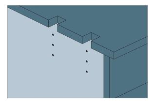
E1. The post is attached to the fascia surface. In order for the post to sit flush against the surface, the floor substrate's overhang may need to be notched prior to post installation.
