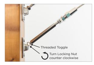
E3. Finish by tightening the Locking Nut on the Threaded Toggle in a clockwise direction until it sits flush with the Tensioning Body or a counter clockwise direction until it sits flush with the fastening plate.
