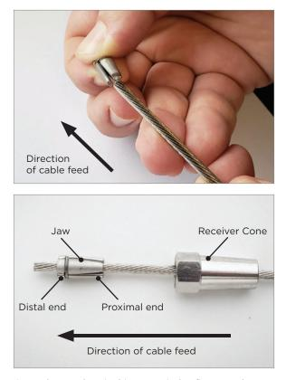
D3. Open the Jaw by pinching your index finger and your thumb on the distal end of the Jaw. Feed the 1/8" cable through the Jaw.
