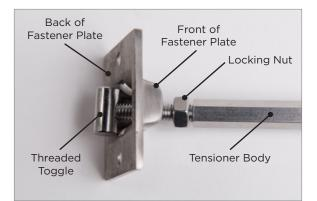
B1. To allow for the Fastener Plate to be securely attached to the end post with screws ensure that the threaded toggle can swivel freely within the base. The Locking Nut may need to be backed away from the front of the Fastener Plate.
