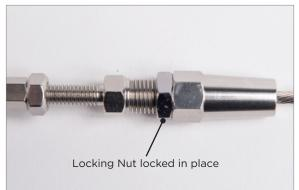
D7. Use a 12mm wrench to turn the Locking Nut in a counter clockwise direction, this will lock the Receiver Cone into place.
