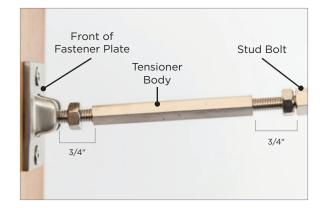
B3. Ensure there is a 3/4" gap between the Fastener Plate and the Tensioner Body as well as a 3/4" gap between the Tensioner Body and the Stud Bolt. Adjust the Hex Shaft on the Threaded Toggle and Tensioning Screw until a 3/4" gap on each side of the Tensioning Body has been achieved.
