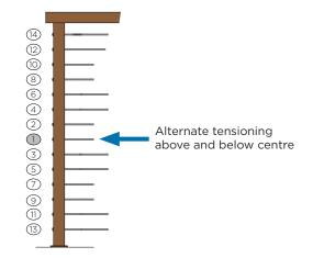
Alternating between cables above and below the center run of cable, tighten until the cable is taut.
