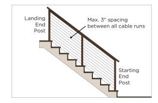
A2. Begin at the lowest cable run of the Starting End Post and run a chalk line to the top of the Landing End Post. Snap and mark the chalk line parallel the slope angle of the stairs. Measure 3" on center perpendicular to the line snapped and sequentially snap and mark a chalk line for the cable runs above.
