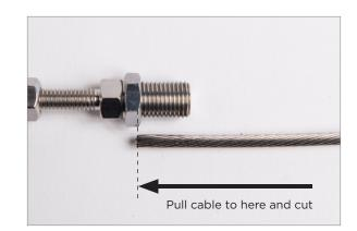
D1. Pull the cable, which is already attached to the non-tensioning fitting on the opposing end post, to the face of the Locking Nut. Measure, mark, and then cut the cable using a cable cutter.
