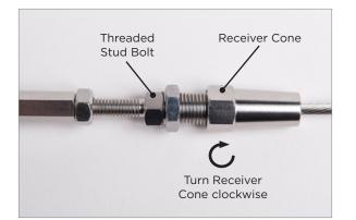
D6. Use a 10mm wrench to hold the Threaded Stud Bolt. Holding the Threaded Stud Bolt will keep it from spinning while the Receiver Cone is being tightened.
