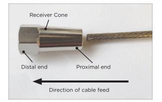
D2. Feed the 1/8" cable through the Receiver Cone from the proximal end.
