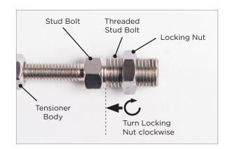
C1. Screw the Locking Nut in a clockwise motion on to the Threaded Stud until the Locking Nut is flush against the Threaded Stud Bolt.
