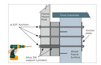
E3. Mount the post and block to the fascia surface using the recommended fasteners for the appropriate frame substrate (see page 5). The support cylinders must be positioned before anchor installation on the lowest hole. The anchor holds the post and block together once tightened.
