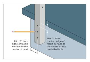
D2. Begin with the end post, determine the placement ensuring that minimum edge distances are maintained. Mark holes to be drilled.
