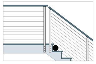
NOTE: A 6" sphere should not pass through the landing of the stair and the first intended cable run.
