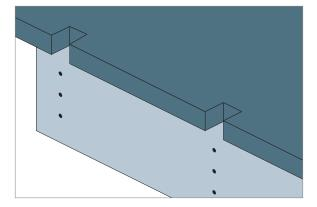
E1. The post is attached to the fascia surface. In order for the post to sit flush against the surface, the floor substrate's overhang may need to be notched prior to post installation.
