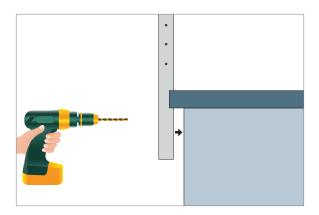
E2. Mount the post to the fascia surface using the recommended fasteners for the appropriate frame substrate (see below).
