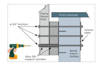
E3. Mount the post and block to the fascia surface using the recommended fasteners for the appropriate frame substrate (see page 4). The support cylinders must be positioned before anchor installation on the lowest hole. The anchor holds the post and block together once tightened.
