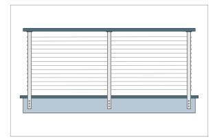
F1. Handrail must be mounted prior to cable infill installation. Complete the railing by adding infill. Please refer to <u>Installation Instructions for Metal Posts</u> <u>on Level Runs, Tensioning</u>
