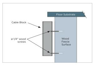
E2. Attach the cable block to the fascia surface using  $\emptyset 1/4''$  wood screws (supplied by others).
