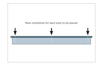
D1. Using 48" on center as the maximum spacing between posts, determine where each post will be placed and mark their centerlines. Do this for the entire level run of your project. Spans greater than 48" will allow excess room for cable deflection.
