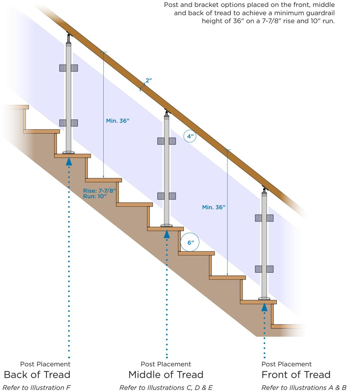
Bezdán Stainless pre-drilled and pre-assembled posts and top mount brackets provide a variety of off-the-shelf solutions for your projects. See the different post and bracket configurations on page 2.
