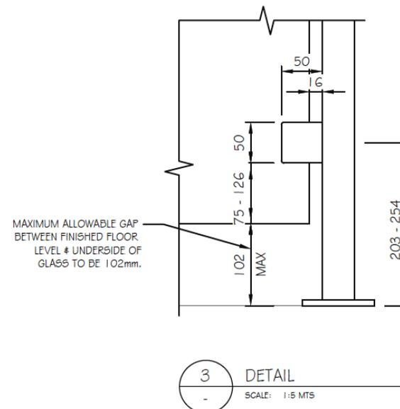
FOR THE INTERIOR INSTALLATION SHOWN, THE BEZDAN STAINLESS STEEL POST & RAIL SYSTEM MEETS THE REQUIREMENTS OF THE RELEVANT IBC 2018 AND IRC 2018 CLAUSES BELOW.
