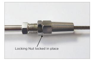
D3. Use a 12mm wrench to turn the Locking Nut in a counter clockwise direction, this will lock the Receiver Cone into place.
