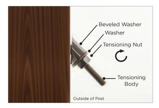
B2. From outside of post slide on the Beveled Washer followed by the Washer. Screw tensioning nut onto the Tensioning Body in a clockwise direction. Use an 11mm wrench to fully tighten the Tensioning Nut.
