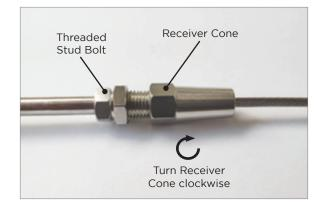
D2. Use a 10mm wrench to hold the Threaded Stud Bolt. Holding the Threaded Stud Bolt will keep it from spinning while the Receiver Cone is being tightened.
