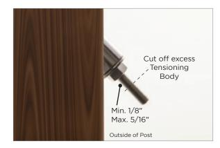
E1. The Tensioning Body can be cut to a minimum length of 1/8" with a maximum exposed length of 5/16" to allow the Acorn Nut to be affixed.
