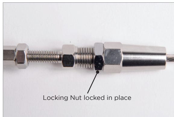
D4. Use a 12mm wrench to turn the Locking Nut in a counter clockwise direction, this will lock the Receiver Cone into place.
