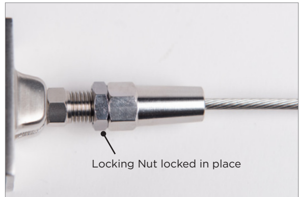
C3. Use a 12 mm wrench to turn the Locking Nut in a counter clockwise direction, this will lock the Receiver Cone into place.
