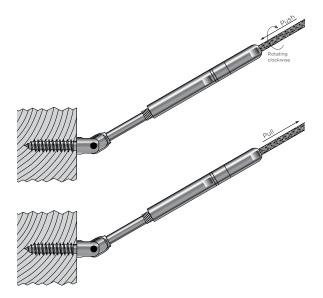
13. Tension cable by holding Push-Lock® body at 3/8" wrench flat nearest cable (do not let this section rotate while cable is inserted) and rotating female threaded section of fitting with a 3/8" open-end wrench onto threads.
