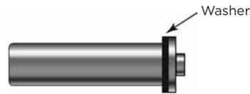
2. Rotate the Pull-Lock® fitting clockwise as you push it onto the cable. If the cable begins to "unravel," you are rotating the fitting in the wrong direction.
