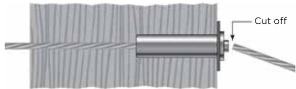
2. Twist the cap onto the lip of the Pull-Lock® fitting.
