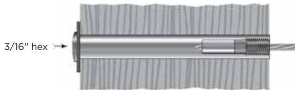
The swaging stud will be pulled into the Receiver by rotating the Receiver clockwise.
