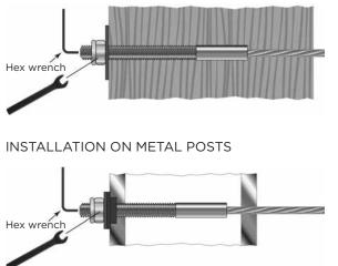
2. Tension all cables to desired amount in sequence, beginning with the center cables, moving up and down toward the top and bottom. As you tension each cable, give it a sharp pull downward mid-span to help set the wedges, then re-tension as necessary in the same sequence. Be aware that the cable may move as much as 3/16" toward the tensioning terminal as the wedges seat.
