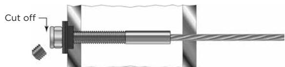
2. Twist the cap over the locknut.
