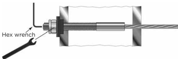
2. Tension all cables to desired amount in sequence, beginning with the center cables, moving up and down toward the top and bottom. As you tension each cable, give it a sharp pull downward mid-span to help set the wedges, then re-tension as necessary in the same sequence. Be aware that the cable may move as much as 3/16" toward the tensioning terminal as the wedges seat.
