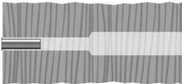
2. If using metal posts, start by inserting the plastic stud bushing into the pre-drilled hole in the post. Slide the stainless steel washer onto the threaded stud (smaller for metal post, larger for wood) and start the brass locknut onto the threads as far as possible by hand. Feed the cable through the end post, pulling the threaded stud into place.
