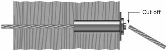
4. Twist the cap onto the lip of the Pull-Lock® fitting.
