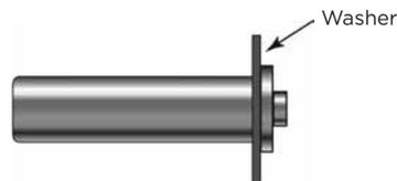
2. Rotate the Pull-Lock® fitting clockwise as you push it onto the cable. If the cable begins to "unravel," you are rotating the fitting in the wrong direction.
