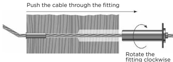
Note: If you have trouble inserting the cable into the fitting, it may be because the locking wedges have become stuck. This is not a defect!
