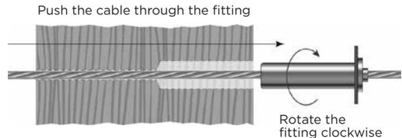
Note: If you have trouble inserting the cable into the fitting, it may be because the locking wedges have become stuck. This is not a defect!
